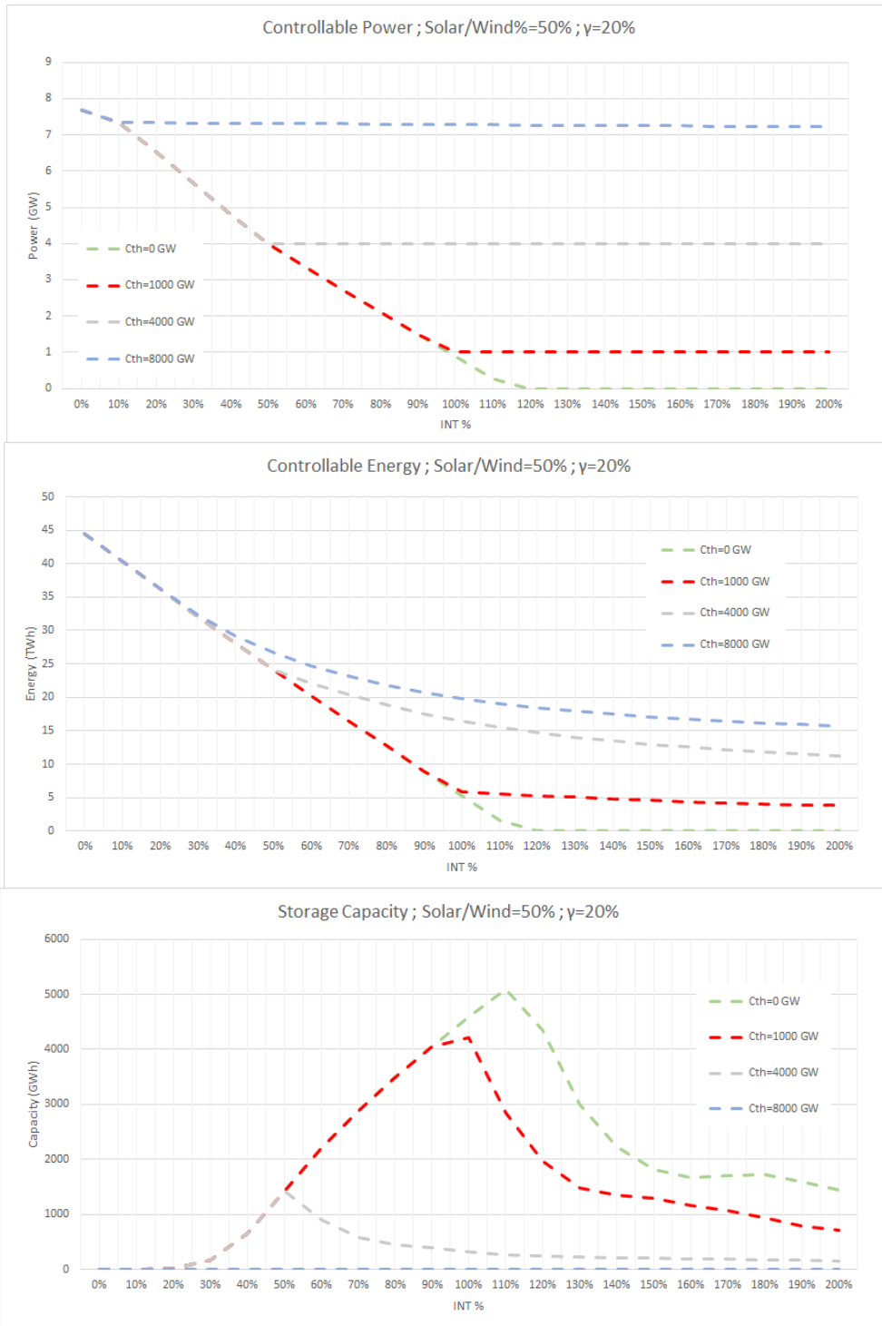
Figure 22 Required controllable energy (a), maximum required controllable power (b), storage capacity (c) as a function of various energy introduction scenarios (%INT) for a 50% solar/wind mix with storage, for various values of Cth. \gamma = 20\% .
